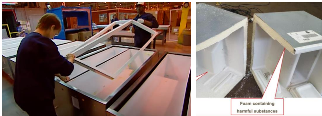
Figures D3 and D4. Refrigerator walls assembly for foam injection, Cut refrigerator walls where the foam can be seen. Retrieved on July 1 st , 2022, from: https://www.youtube.com/watch?v , https://transparency-partnership.net/system/
