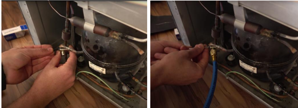
Figures D5 and D6. Man installs a piercing valve. Man re-charges refrigerant into the cooling system through the piercing valve. Retrieved on July 1 st , 2022, from: https://www.youtube.com/watch?v=j
