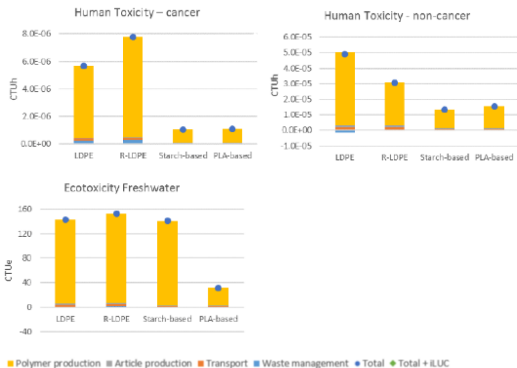
Figure C2 Comparison of environmental impacts through the Life Cycle of one hectare mulch films for the following scenarios: LDPE, recycled LDPE, starch based biopolymer and PLA based biopolymer. Impact expressed in Comparative Toxicity Units (CTU), from [36].
